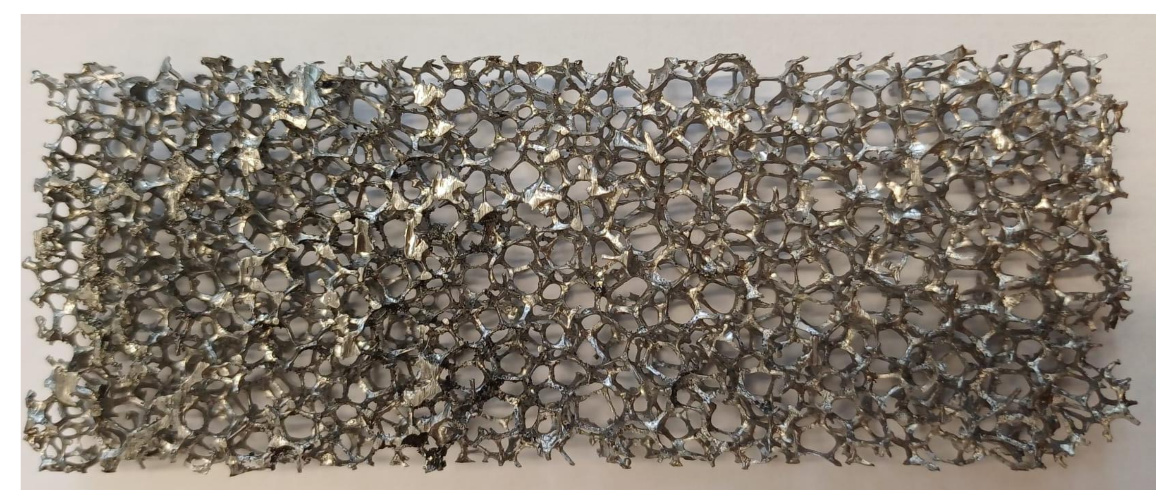
Alternative Structure: Metal Foam
