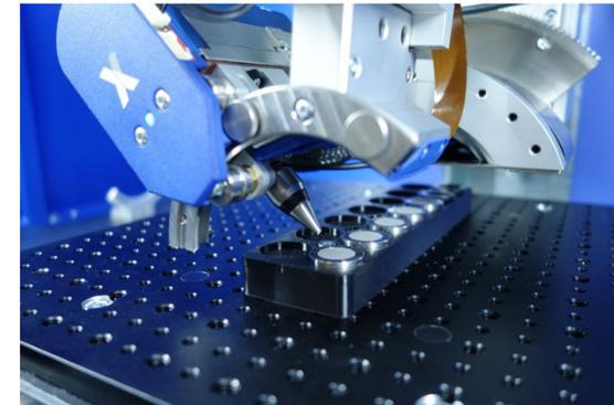
Measurement of residual stresses with x-ray diffraction
