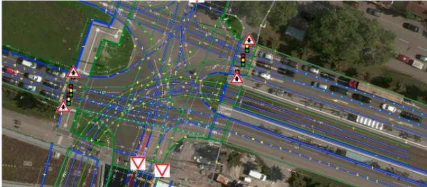
Figure 1: Example of a vectorized map with road boundaries, lane boundaries and traffic signs
